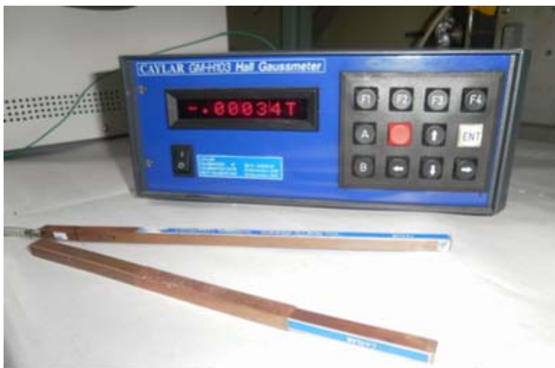
Figure 21: Caylar GM-H103 Hall Gaussmeter.
